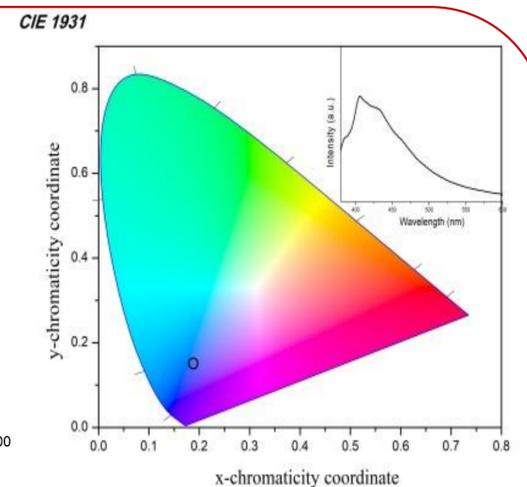
Fig. 4. CIE coordinates of the mechanochemically synthesized ZnMoO<sub>4</sub>
