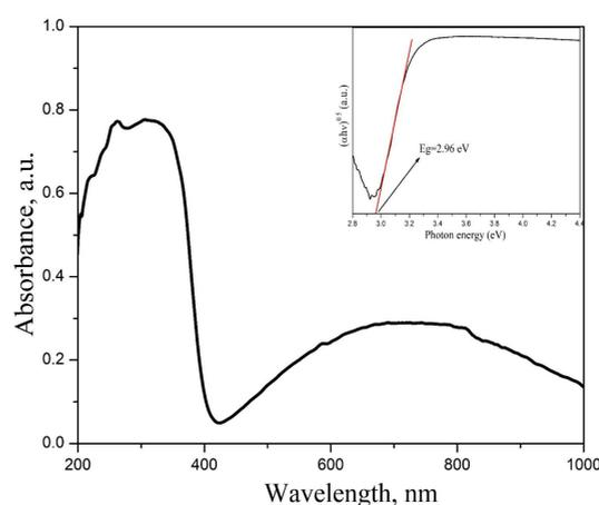
Fig. 3. The absorption spectrum of mechanochemically synthesized ZnMoO<sub>4</sub>
