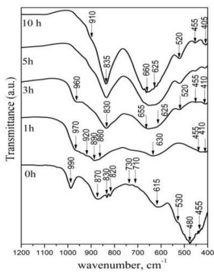
Fig. 2. IR spectra of the mixture of initial ZnO and MoO<sub>3</sub> mechanochemically activated for different milling times.
