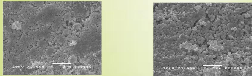
SEM images of tablets heated at 900 °C for 40 hours top view:  $\text{LaCo}_{0.8}\text{Ni}_{0.1}\text{Fe}_{0.1}\text{O}_3$  (left) obtained at normal pressure and (right) a sample obtained under high-oxygen pressure  $\text{LaCo}_{0.8}\text{Ni}_{0.1}\text{Fe}_{0.1}\text{O}_3$ .
